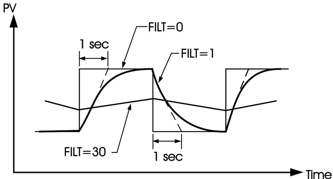
Figure 3.8 Filter Characteristics
