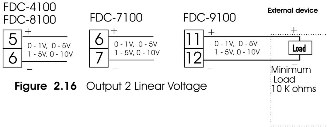
**Figure 2.16** Output 2 Linear Voltage
