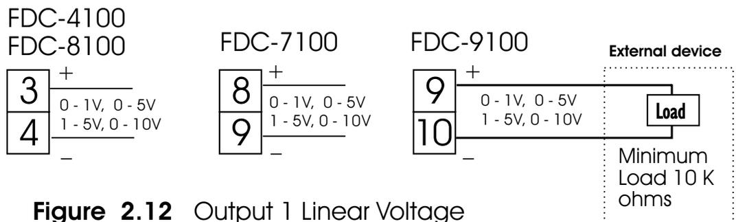
**Figure 2.12** Output 1 Linear Voltage
