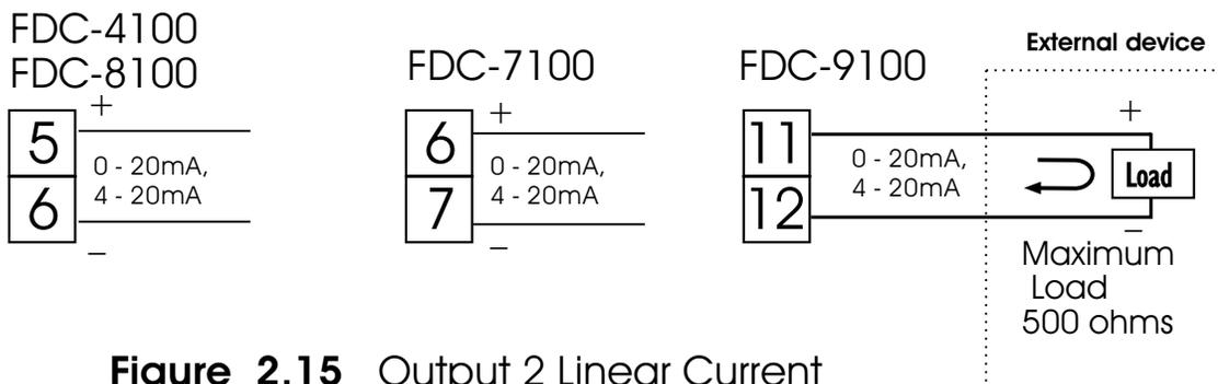
**Figure 2.15** Output 2 Linear Current
