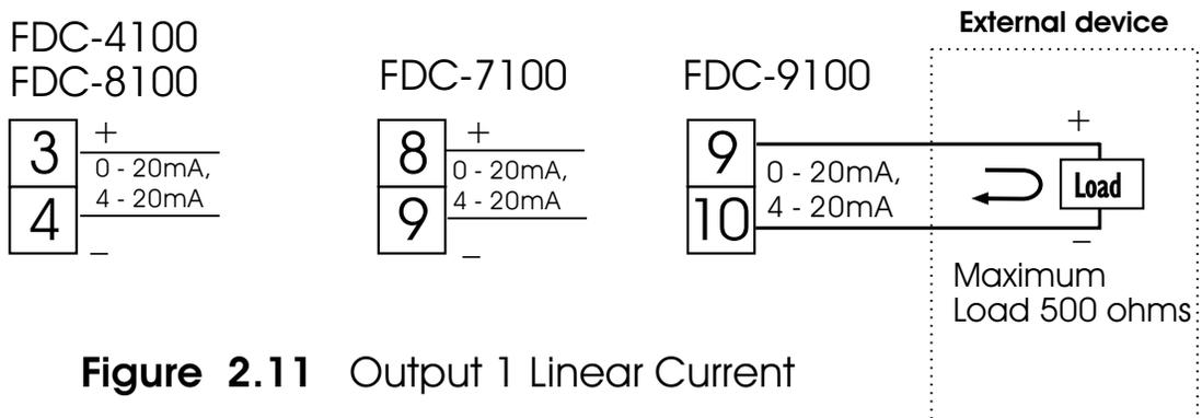
**Figure 2.11** Output 1 Linear Current
