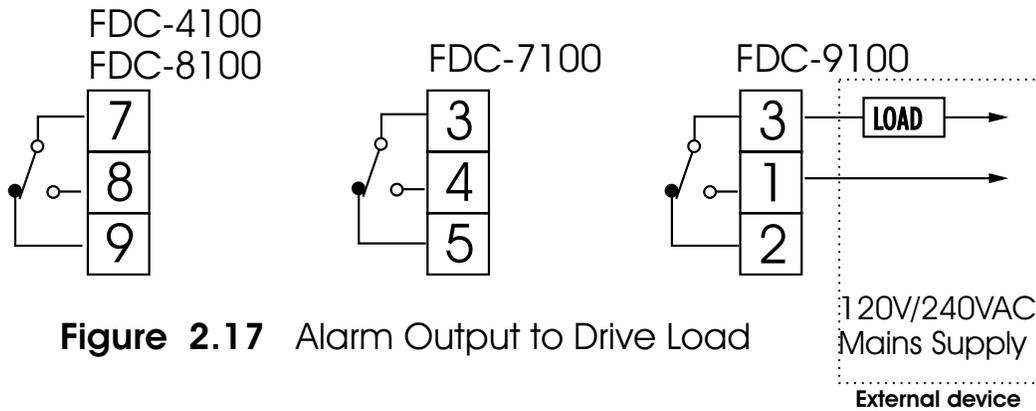
**Figure 2.17** Alarm Output to Drive Load
