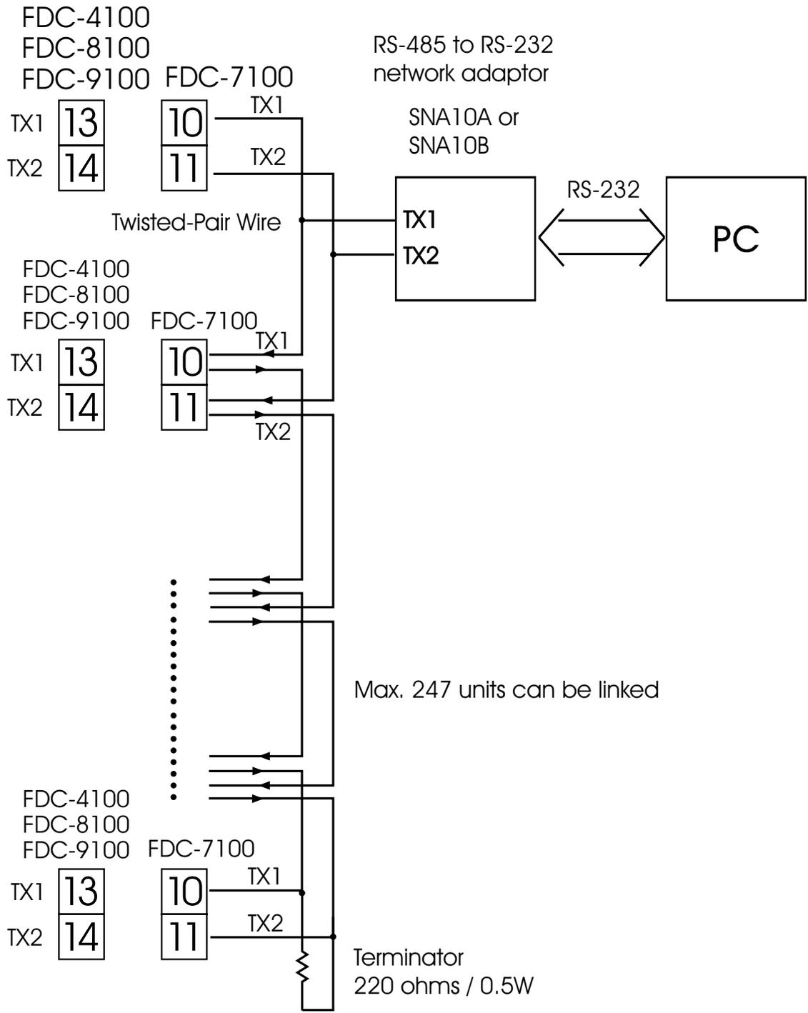
**Figure 2.19** RS-485 Wiring
