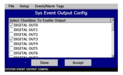
For each output that is to be assigned to the event, place a check in the checkbox next to the digital output. Once all selections have been made, press the 'Accept' button to assign the outputs to the event, and then press 'Done' button to return to the System Event Configure screen. If you do not press 'Accept' prior to leaving the event output configuration screen, any changes will be ignored.
