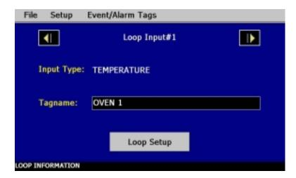
The loop input number in the upper right of the display, shows the current loop selected for configuration. The left and right scroll buttons adjacent to the loop input number, allow the user access each loop in the system, by pressing left or right to go to the previous or next loop.
