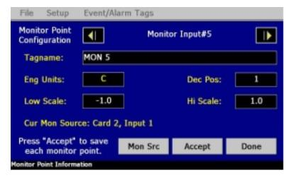
The monitor input number in the upper right of the display, shows the input selected for configuration. The left and right scroll buttons adjacent to the monitor input number, allow the user to access each monitor point in the system by pressing left or right to go to the previous or next input.
