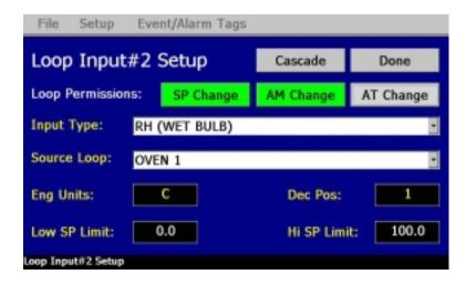
The **Input Type** selection is used to set the input type of the loop. There are three selections available for the type of input that can be used with the Orion-M:
