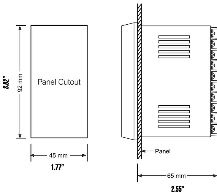
Figure 2.1 Mounting Dimensions
