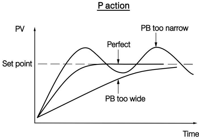
Figure 3.7 Effects of PID Adjustment
