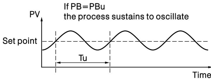
Figure 3.6 Critical Steady State
