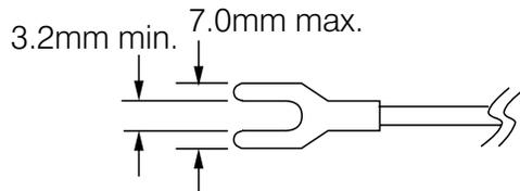
Figure 2.2 Lead Termination
