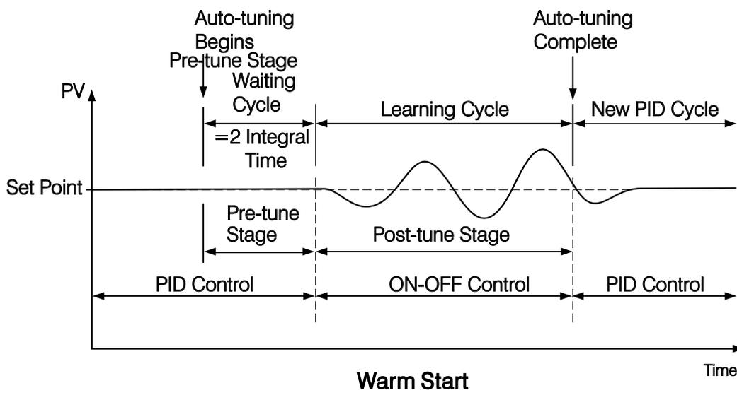
If the auto-tuning begins near the set point ( warm start ), the unit passes the warm-up cycle and enters the waiting cycle. Afterward the procedures are same as that described for cold start.
