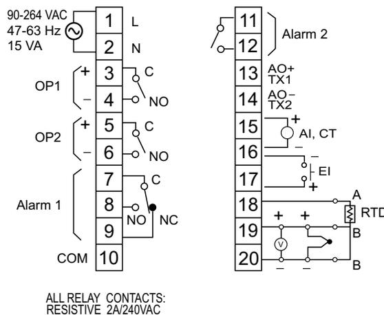
Figure 2.3 Rear Terminal Connection Diagram
