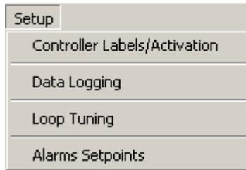
The "**Controller Labels/Activation**" menu under the "Setup menu allows the user the enable/disable any controller attached to the PC. This can be done in any order (Controller addresses do not have to be in sequence for the system to work properly)
